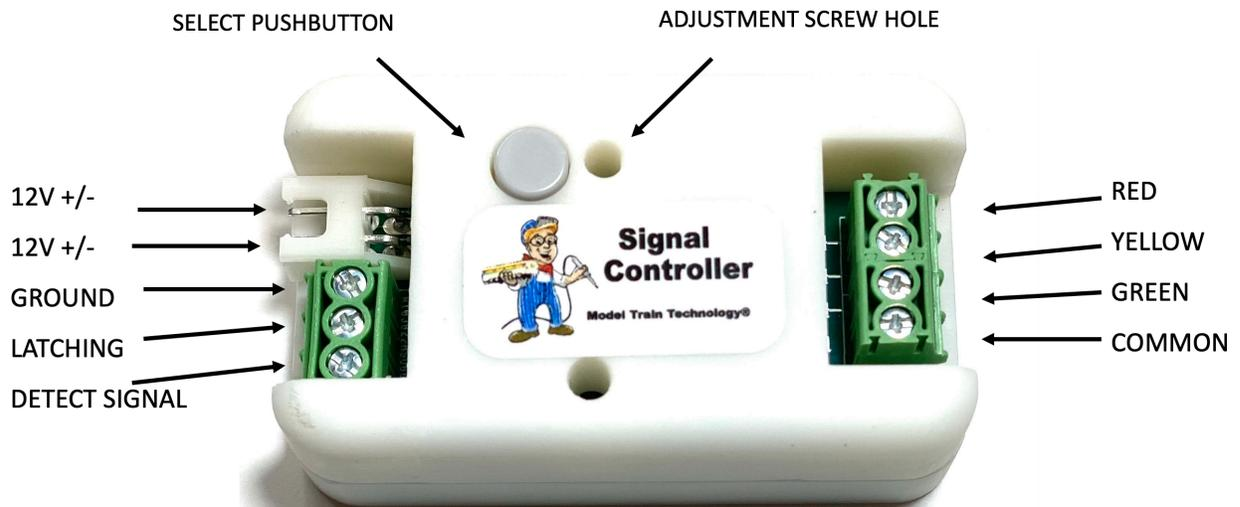
When you plug in power the blue internal LED will light. The green LED or FIBER output will light.
