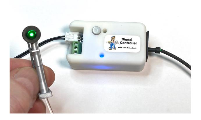
HO Scale: Simply plug the fiber into the Controller Manifold hole (no pin required)
