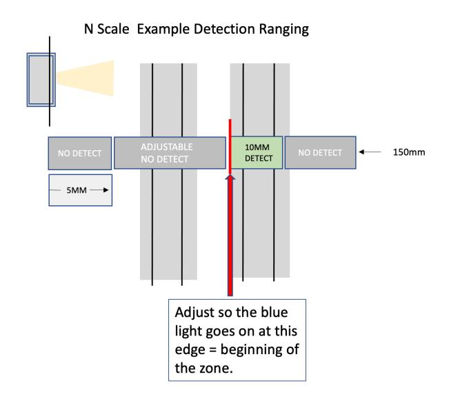
Keep in mind that the trim pot rotation is 300 degrees which allows adjustment over 145mm. When you are adjusting the range in N Scale it only takes a small amount of rotation to move 10mm.
