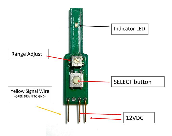
The Mile Marker version of the Precision Detector does not have an adjustable trim to set the Detect timeout. Instead, you use the Select button to choose between Immediate (no timeout) and 15, 30, 45 and 60 Seconds)
