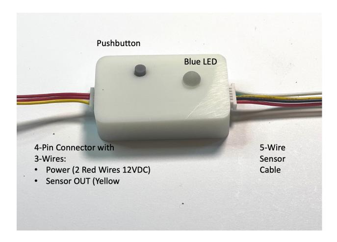
Plug the sensor into the 5-wire connector BEFORE turning the power on – otherwise it will not start or calibrate.
