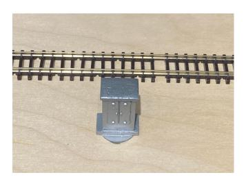
Slide the electrical box cover onto the circuit board – again carefully using the slots on the inside of the box to align with the board.
