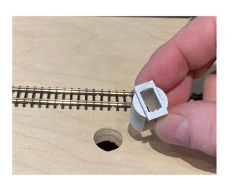
There are two sets of slots in the plug, one for a low mount and another for a high mount of the sensor.
