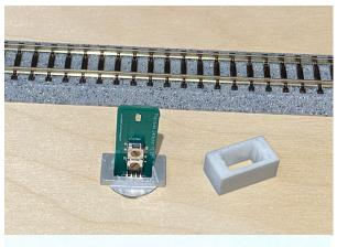
If the Precision Sensor is within 2" of the track, the shorter set up of the sensor will work fine and the spacer may not be needed.
