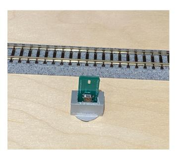
Slide the space collar onto the circuit board just as you did with the plug.
