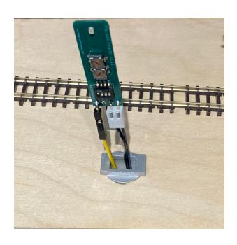
Only plug power into the two closely adjacent pins. The lone third pin is for the yellow sensor wire.
