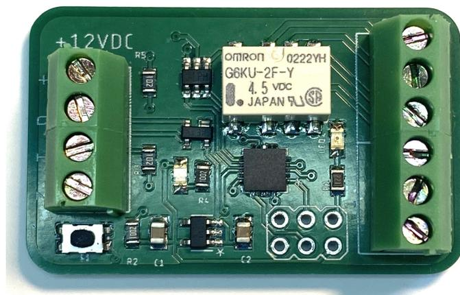
Our Latching relay was upgraded and renamed to SMART Relay. The behavior of this relay can be changed by pushing the onboard pushbutton. The SMART switch is part of some non-computer layout animation projects that we're working on. Here is a short video on how it works:
