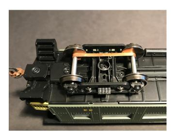
The width of the board is 11.5mm. In a few situations you may have a better fit at about 11mm. For example, this was the case for the Amtrak Skylight car. It's perfectly ok to sand down the edge of the board up to a total of about 1mm. Use your good judgement on this. The
