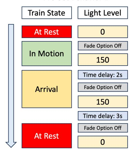
Note: light levels and time can be set from 0 to 255. 100% on is 255.
