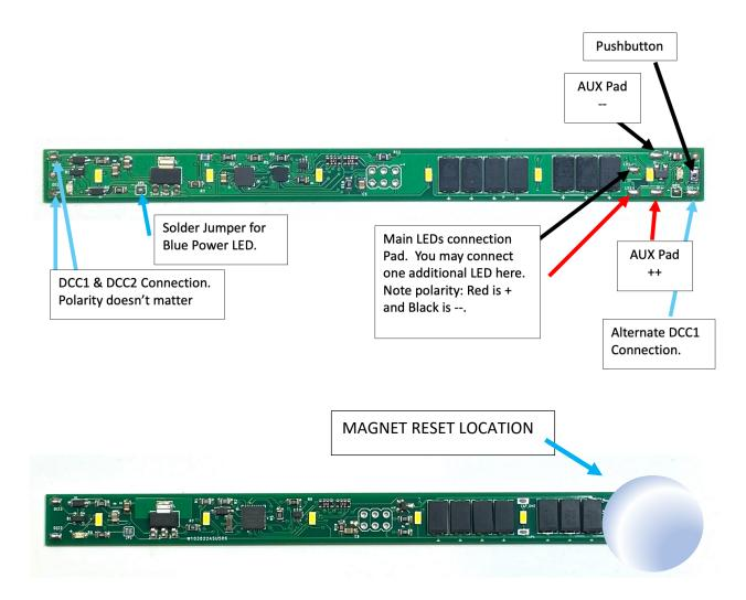
We've changed the board so that both the blue power LED and the red read LED each have a solder pad (JP1 and JP2) that we solder/connect during manufacturing and testing.
