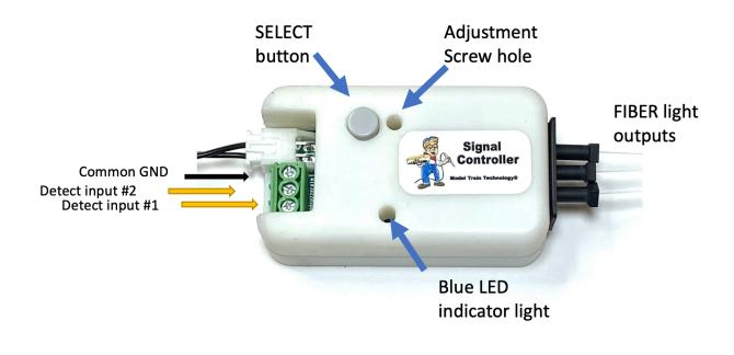
When you plug in power the blue internal LED will light. The CLOSED or green side of each FIBER output will light.
