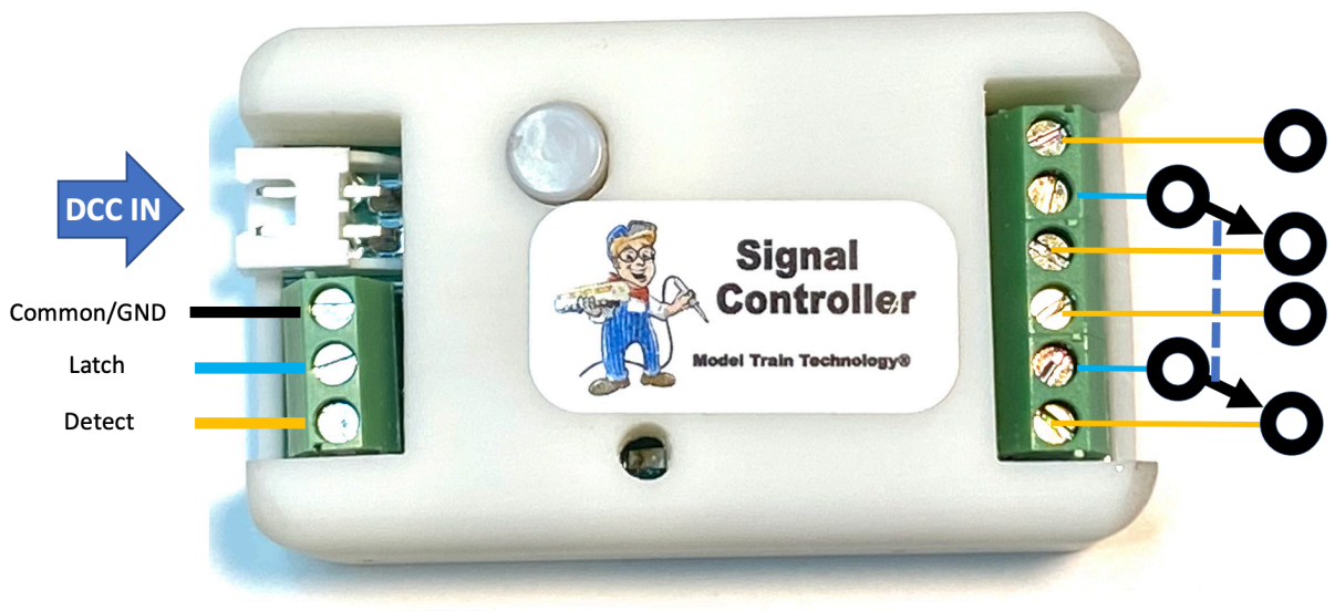
Relay Shown in OFF (Closed) position
